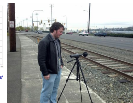
A Distance Education student collects traffic noise L_{eq} data for his ACS 537 Engineering Noise Control class project
